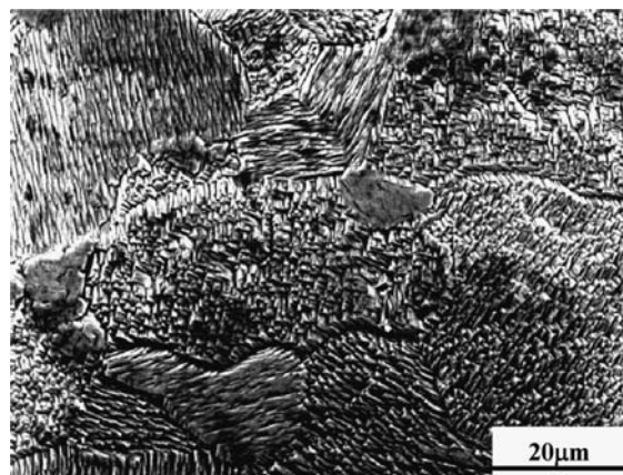
Fig. 4. Morphology of zinc electrodeposited at 25^\circ\text{C} and 10 \text{ mA cm}^{-2} .
